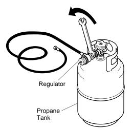
Figure 2 - Connecting Heater to Propane Tank
