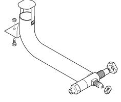
**Burner Assembly Kit - 101864-01** Includes automatic control valve, hardware, and instruction sheet
