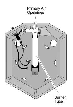
Figure 6 - Bottom View of Heater
