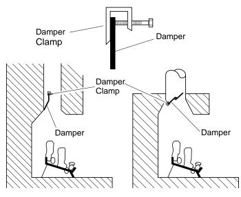
Masonry Fireplace Manufactured Fireplace Figure 10 - Attaching Damper Clamp
