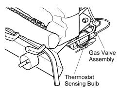
Figure 31 - Location of Gas Valve Assembly and Thermostat Sensing Bulb
