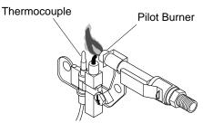
Figure 26 - Incorrect Pilot Flame Pattern
