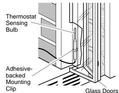
Figure 36 - Installing Thermostat Sensing Bulb behind Glass Doors
