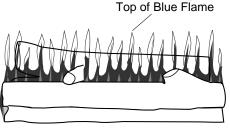
Figure 28 - Incorrect Front Burner Flame Pattern
