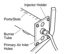
Figure 29 - Injector Holder On Outlet Burner Tube
