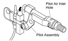
Figure 30 - Pilot Inlet Air Hole
