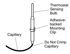
Figure 37 - Positioning the Thermostat Sensing Bulb in the Vertical Position with the Capillary at the Bottom
