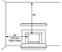
Figure 4 - Minimum Clearance to Wall and Ceiling Continued
