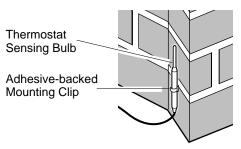
Figure 34 - Locating Thermostat Sensing Bulb on Masonry Fireplace
