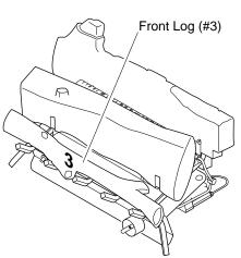
Figure 19 - Installing Front Log
