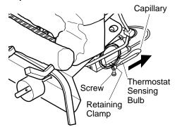
Figure 33 - Removing Thermostat Sensing Bulb
