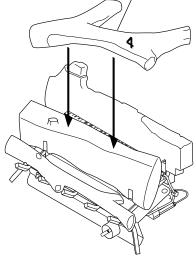
Figure 20 - Installing Top Log
