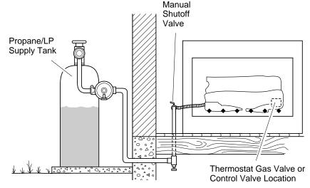
Figure 16 - Checking Gas Joints
