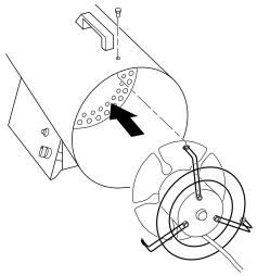
Figure 10 - Replacing Motor and Fan Guard into Heater
