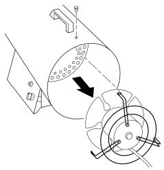
Figure 7 - Removing Motor and Fan Guard from Heater
