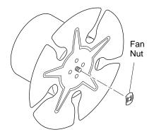
Figure 8- Removing Fan Nut from Motor Shaft
