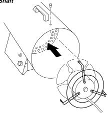
Figure 13 - Replacing Motor and Fan Guard into Heater
