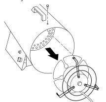
Figure 11 - Removing Motor and Fan Guard from Heater
