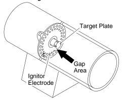
Figure 16 - Clearance between Ignitor Electrode and Target Plate
