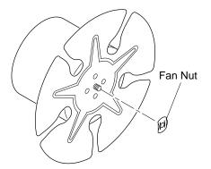
Figure 12 - Removing Fan Nut from Motor Shaft
