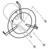
Figure 9 - Removing or Attaching Fan Guard from Motor
