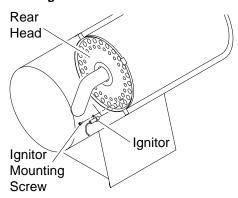
Figure 15 - Removing Ignitor Mounting Screw and Ignitor
