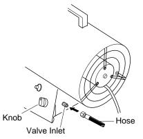
Figure 4 - Hose and Inlet Connector
