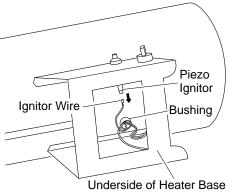
Figure 14 - Removing Ignitor Wire from Piezo Ignitor
