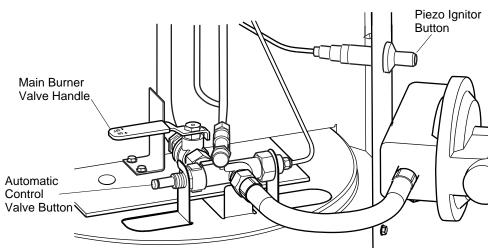
Figure 3 - Main Burner Valve Handle, Automatic Control Valve Button, and Piezo Ignitor Button Locations, With Regulator Installed
