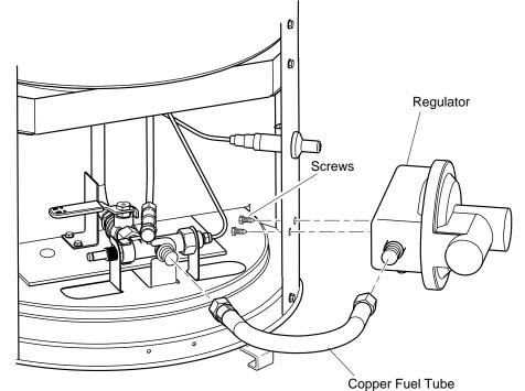
Figure 2 - Installing Regulator
