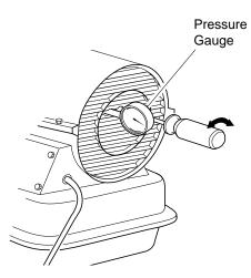
Figure 8 - Adjusting Pump Pressure
