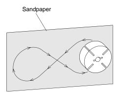
Figure 19 - Sanding Rotor
