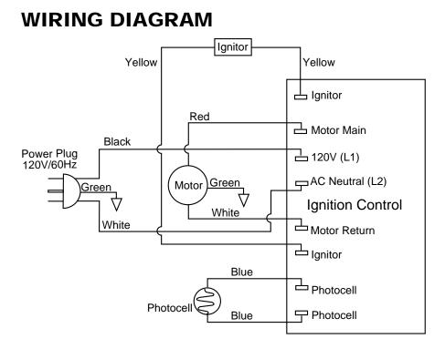
Figure 21 - Wiring Diagram
