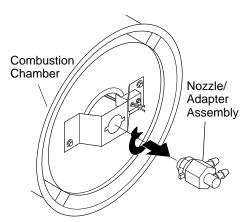
Figure 14 - Removing Nozzle/Adapter Assembly
