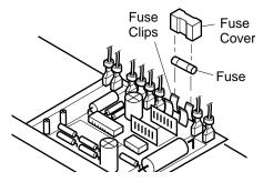
Figure 20 - Replacing Fuse
