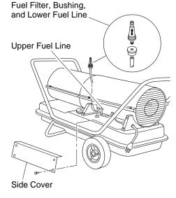
Figure 9 - Fuel Filter Removal
