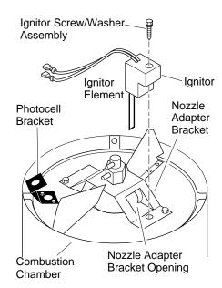
Figure 11 - Ignitor Replacement
