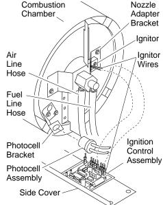
Figure 10 - Disconnecting Ignitor Wires from Ignition Control Assembly
