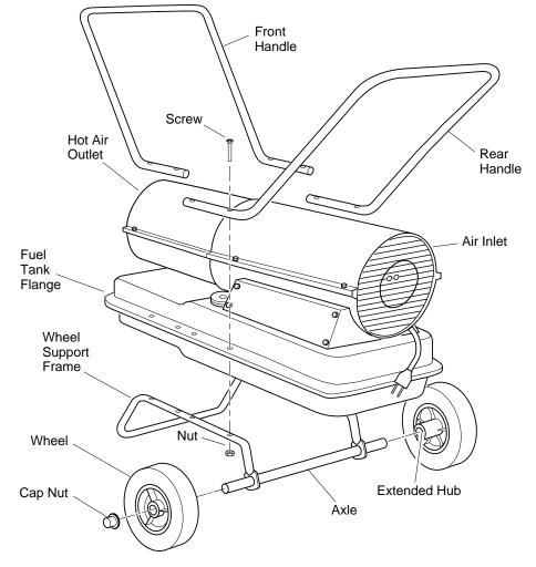
Figure 1 - Wheel and Handle Assembly
