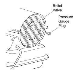
Figure 7 - Pressure Gauge Plug Removal
