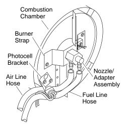
Figure 13 - Removing Air and Fuel Line Hoses (155,000 Btu/Hr Models Only)
