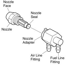
Figure 15 - Nozzle and Nozzle Adapter
