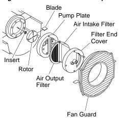
Figure 15 - Rotor Location
