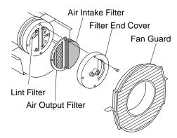
Figure 5 - Air Output, Air Intake, and Lint Filters
