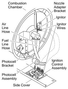
Figure 9 - Disconnecting Ignitor Wires from Ignition Control Assembly (see Wiring Diagram, Figure 18 or 19 appropriately, page 10)
