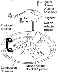
Figure 10 - Ignitor Replacement
