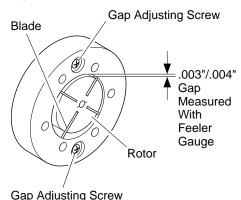
Figure 16 - Gap Adjusting Screw Locations
