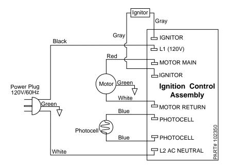
Figure 19 - Wiring Diagram for Heaters Using 102350-01 Ignition Control Assembly
