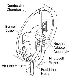
Figure 12 - Removing Air and Fuel Line Hoses
