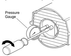
Figure 7 - Adjusting Pump Pressure
