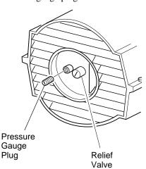
Figure 6 - Pressure Gauge Plug Removal
