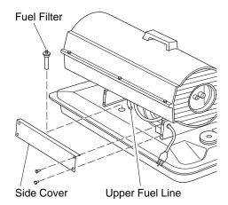
Figure 8 - Fuel Filter Removal
