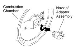
Figure 13 - Removing Nozzle/Adapter Assembly
