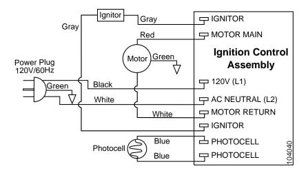
Figure 18 - Wiring Diagram for Heaters Using 104040-02 Ignition Control Assembly
