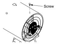
Figure 3 - Removing Screw from Top of Fan Guard
