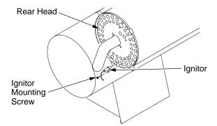
Figure 15 - Removing Ignitor Mounting Screw and Ignitor
