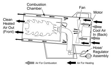
Figure 2 - Cross Section Operational View
