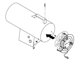
Figure 13 - Replacing Motor and Fan Guard into Heater
