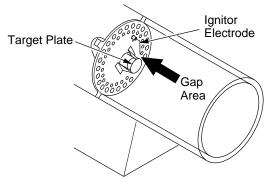
Figure 16 - Clearance between Ignitor Electrode and Target Plate
