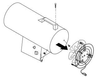
Figure 10 - Removing Motor and Fan Guard from Heater
