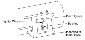
Figure 14 - Removing Ignitor Wire from Piezo Ignitor
