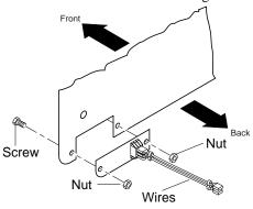
Figure 17 - Switch Plate and Wiring Harness (Switch Plate and Orientation May Vary Depending On Model)
