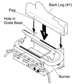
Figure 22 - Installing Back Log (#1)
