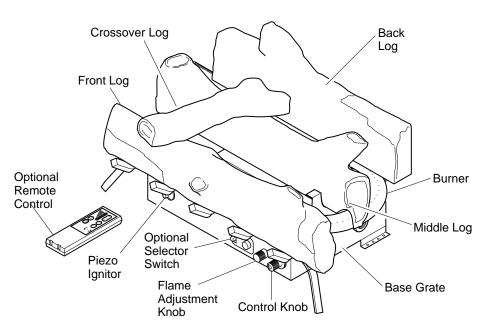
Figure 1 - Vent-Free Gas Log Heater (Logs May Vary By Model)
