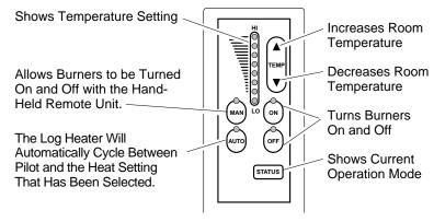
Figure 34 - Thermostat Hand-Held Remote Control Unit Selections
