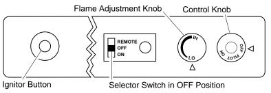
Figure 31 - Control Knob and Ignitor Button Location
