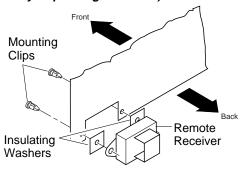
Figure 18 - Installing Remote Receiver
