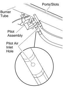
Figure 38 - Pilot Inlet Air Hole
