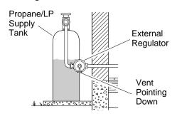
Figure 13 - External Regulator With Vent Pointing Down
