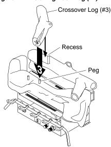
Figure 28 - Installing Crossover Log (#3)
