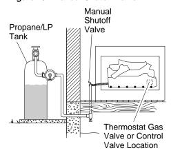
Figure 16 - Checking Gas Joints
