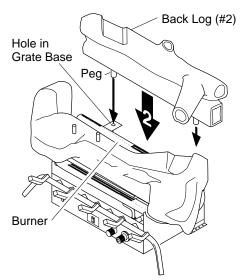
Figure 27 - Installing Back Log (#2)
