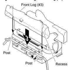
Figure 24 - Installing Front Log (#3)
