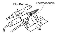
Figure 35 - Correct Pilot Flame Pattern
