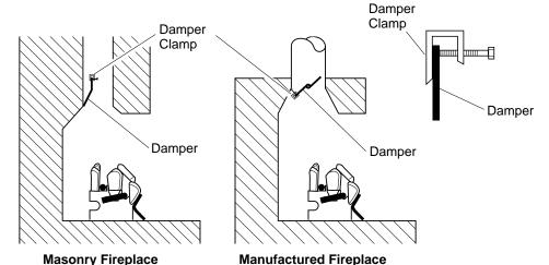
Figure 10 - Attaching Damper Clamp
