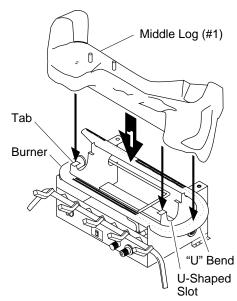
Figure 26 - Installing Middle Log (#1)
