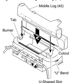
Figure 23 - Installing Middle Log (#2)
