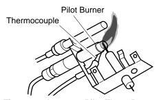
Figure 36 - Incorrect Pilot Flame Pattern
