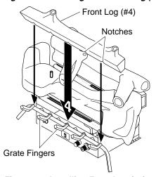
Figure 29 - Installing Front Log (#4)
