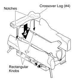
Figure 25 - Installing Crossover Log (#4)
