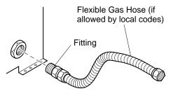
Figure 11 - Attaching Flexible Gas Hose to Heater
