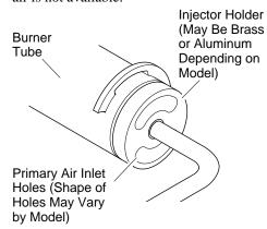
Figure 37 - Injector Holder On Outlet Burner Tube
