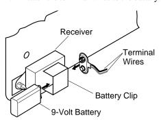
Figure 20 - Installing Receiver on the Back of the Base
