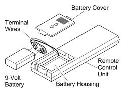
Figure 21 - Installing Battery in Hand-Held Remote Control Unit
