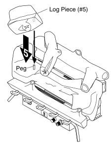
Figure 30 - Installing Log Piece (#5)
