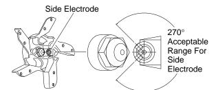
Figure 14 - Acceptable Range For Side Electrode
