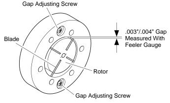
Figure 18 - Gap Adjusting Screw Locations
