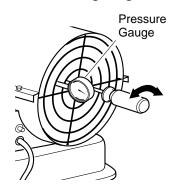
Figure 9 - Adjusting Pump Pressure
