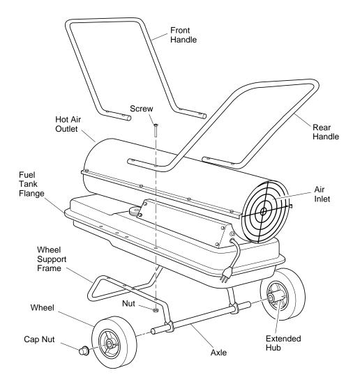
Figure 2 - Wheel and Handle Assembly
