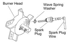
Figure 12 - Spark Plug Removal
