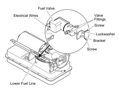
Figure 11 - Fuel Valve Replacement
