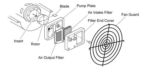
Figure 17 - Rotor Location
