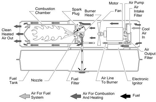
Figure 3 - Cross Section Operational View
