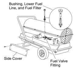
Figure 10 - Fuel Filter Removal
