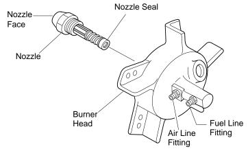
Figure 16 - Removing Nozzle
