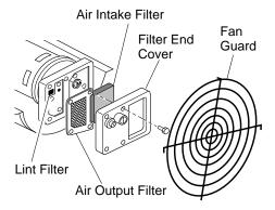
Figure 7 - Air Output, Air Intake, and Lint Filters
