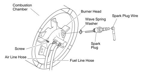
Figure 15 - Removing Burner Head
