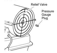
Figure 8 - Pressure Gauge Plug Removal
