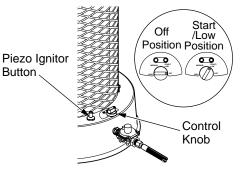
Figure 6 - Control Knob, and Piezo Ignitor Button Locations for Natural Gas Model TC100VRNG
