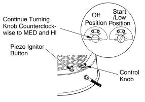
Figure 5 - Control Knob and Piezo Ignitor Button Locations for Propane Model TC100VR
