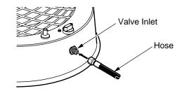
Figure 3 - Hose and Valve Inlet
